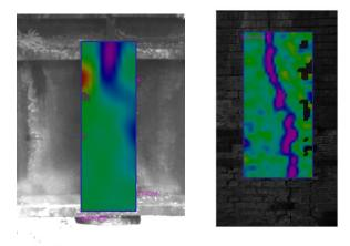
More advanced visualisations of strain are possible by applying a speckle pattern to the component surface.
